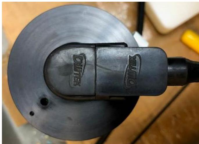
**Figure 3: Correct alignment of LPMBH-6-MP cable connector (-01 configuration)**
